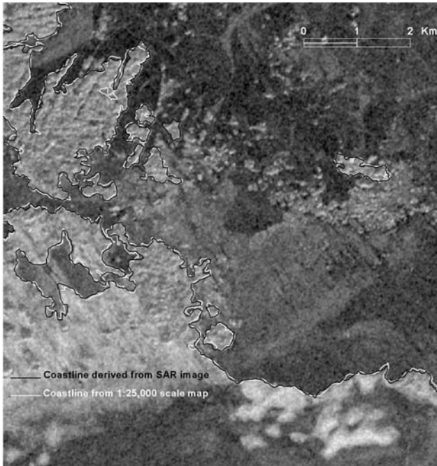
Figure 9. Evaluation of the Radarsat SAR-derived coastlines with reference to a large-scale topographic map (1:25,000).
